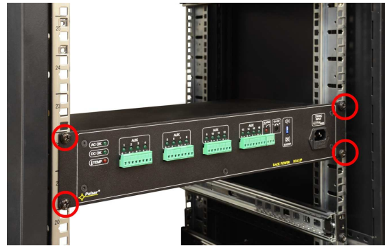
- Secure the enclosure with 4xM6 screws
